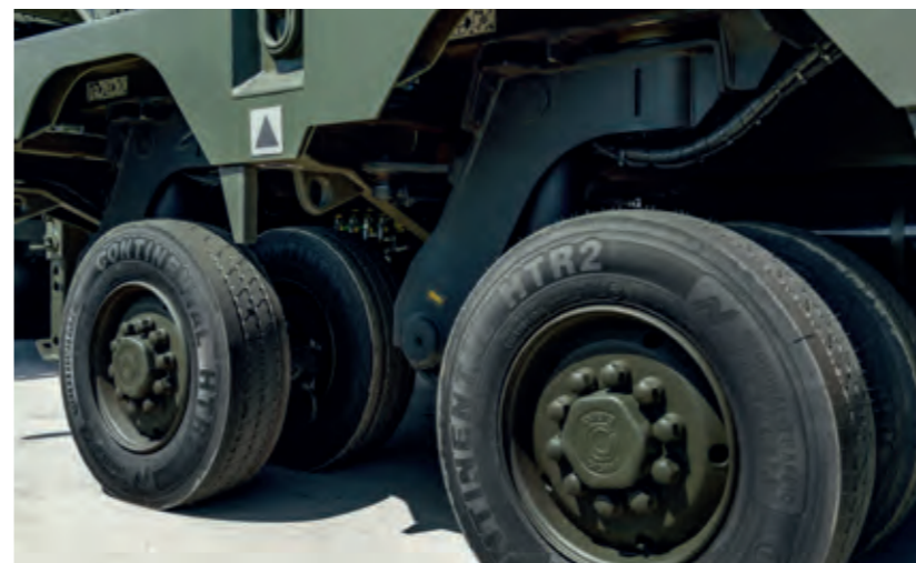
Perfect cooperation of rigid steel structure with independent hydraulic suspension.
