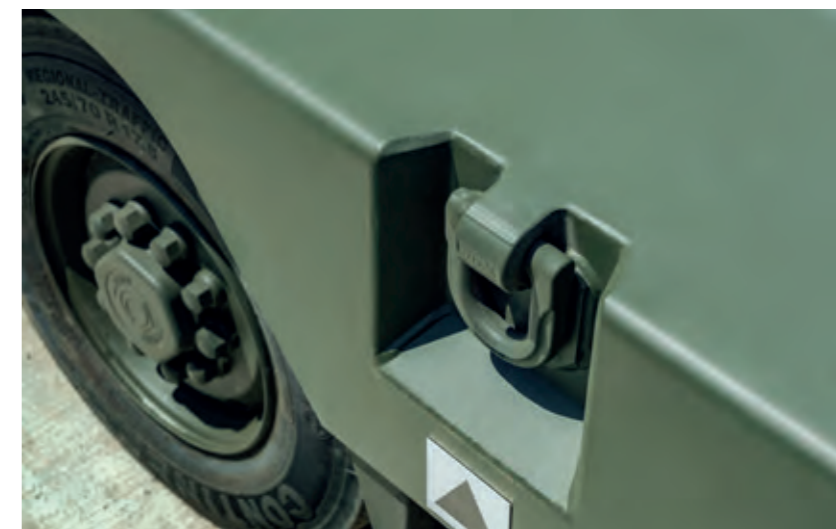
Load fixtures with a force of 20 000 daN
