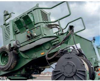
Hydraulic power generator. Spare wheel basket with a crane.
