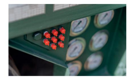
Centralized lubrication system that can be converted to an automatic central system.
