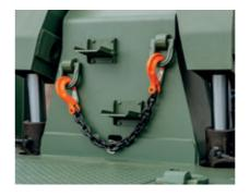
Load securing brackets. Ergonomic access steps.
