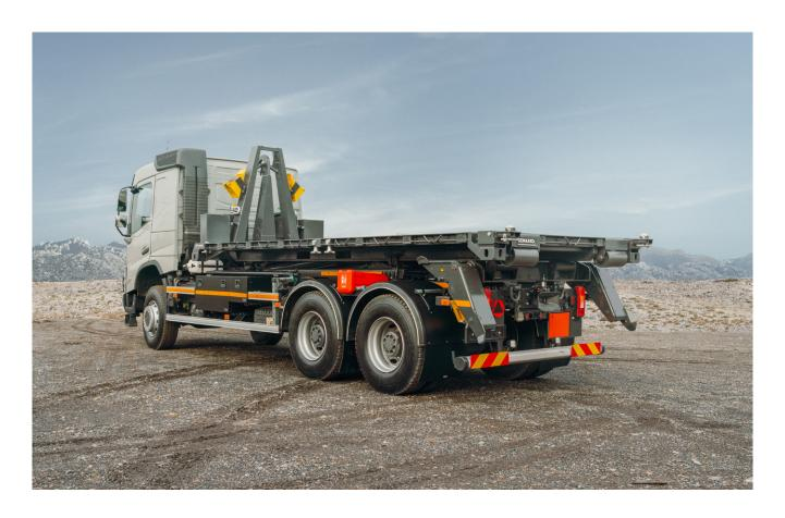
The Flatrack hook loading platform has been specifically designed for use with the HIAB Multilift MK IV lifting device mounted on the Volvo FMX VTN3R vehicle.
